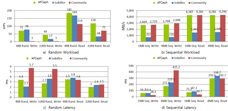
Figure 11: Virtual Machine max performance comparison: SolidFire vs AFCeph vs Community Ceph
